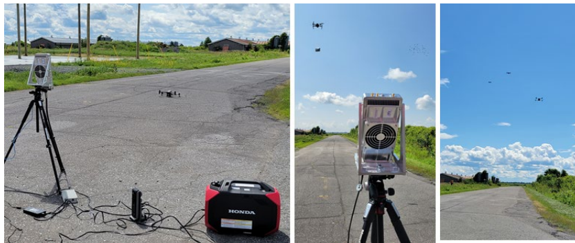
Figure 3: Experimental setup for outdoor drone detection trials.
