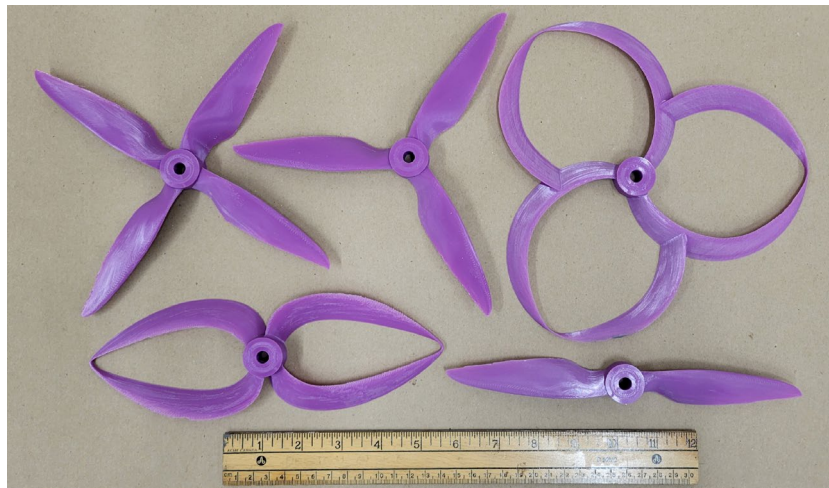
Figure 1: Example of 3D printed toroidal and traditional propeller blades.
